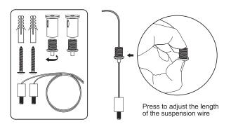
1. Fix hanging rope onto the ceiling.
